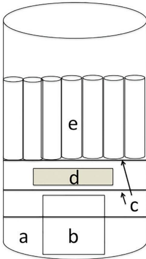
**Fig. 1.** Experimental chambers for controlled RH. Saturated salt solutions (a) were in the bottom of a sealed glass jar, with a section of PVC pipe (b) as a spacer. Metal screening (c) separated the salt solutions, HOBO temperature and RH loggers (d), and experimental vials containing bed bugs (e).
