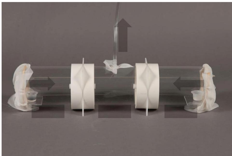
**Fig. 1.** Three-chamber linear olfactometer. The olfactometer was constructed so that the vacuum pump drew air across the treatment and control cups and into the middle chamber, where 20 gravid females were introduced. Cups containing test or control materials were placed on a small shelf at the end of each side chamber. Chambers were connected by 6-cm-long (1-cm-inner diameter) tubes extending 3 cm into both the side chamber and the middle chamber.
